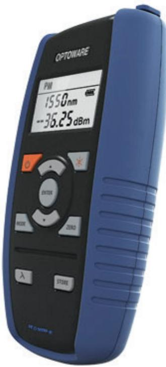
Auto 1nm resolution  $\lambda$  detection and power measurement
