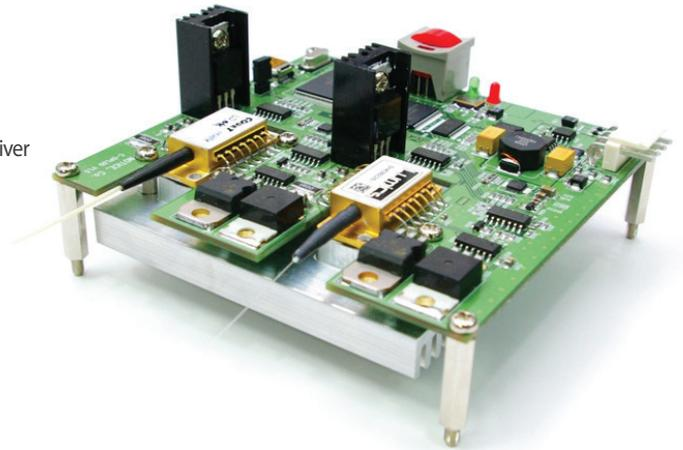
The Dual Pump LD Driver (DPLDD) module is an efficient module which can drive various kinds of pump laser diode for the pumping source of fiber laser, EDFA and ASE broadband source. This module can be used as the high power LD driver for SLED sources, SOA modules and fiber laser seed source LDs and also be used as the driver for driving the different two kinds of LD individually in one board.
