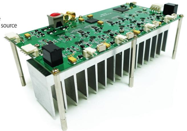
The High Power LD Driver (HPLDD) module is an efficient module which can drive multi-channel high power laser diodes for the pumping source of fiber laser, optical amplifier and industrial laser applications. This module can accommodate up to four laser diodes which can be driven to output various arbitrary shapes of pulse individually
